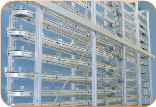
The Alpine Conveyor is a compact spiral configuration commonly used as an accumulation or buffer zone in between machines or as a process step for cooling or drying. It is also used for line balancing and for repair and maintenance purposes.
